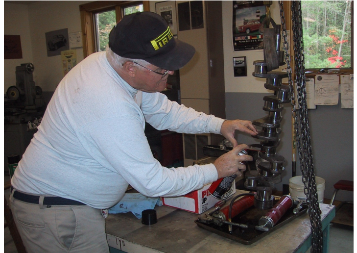
Cleaning Out the Oil Passages in the Crankshaft
